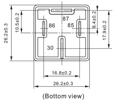
Remark: Terminal vertical deviation tolerance is 0.3mm.
